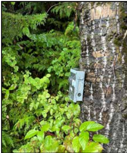
Trail counters provide critical data to understand the amount of traffic a trail gets on any day or hour of the year. Data can help determine and prioritize trail projects.
